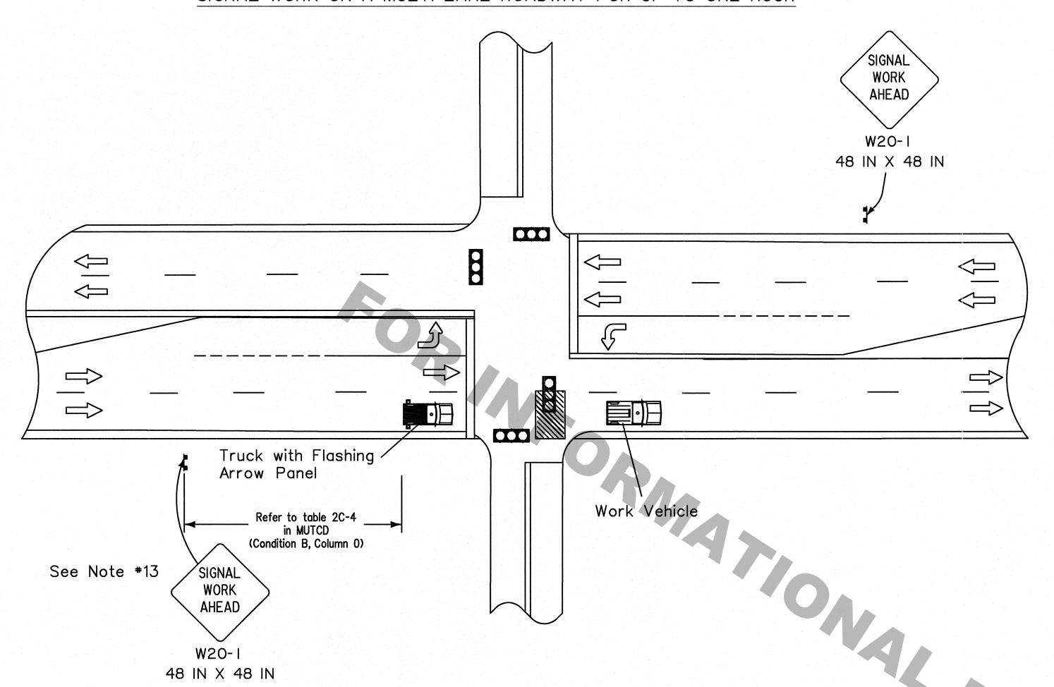
SIGNAL WORK ON A TWO-LANE TWO-WAY ROADWAY
